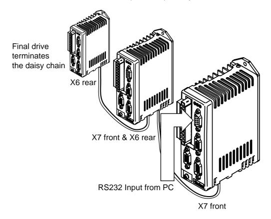
Figure 3-20. RJ45 RS232 Daisy Chain Connections
